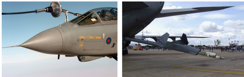
Figure 1: Refuelling methods: (Left) probe-and-drogue and (Right) boom [1]
